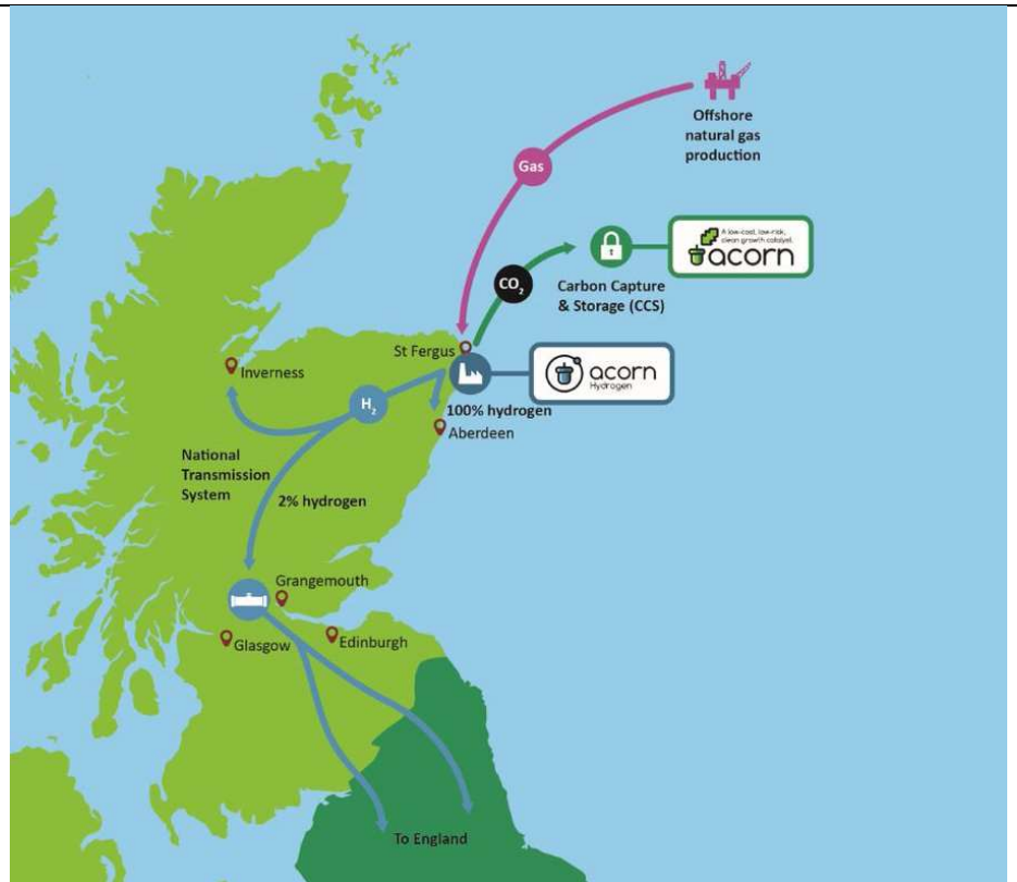
Image 2 –Phase 2 of the Acorn Project. CCS supporting low-carbon hydrogen production at St Fergus gas terminal. The image shows how this can be blended into the current gas network at 2% and potentially at 100% percent to supply the Aberdeen Vision project.
