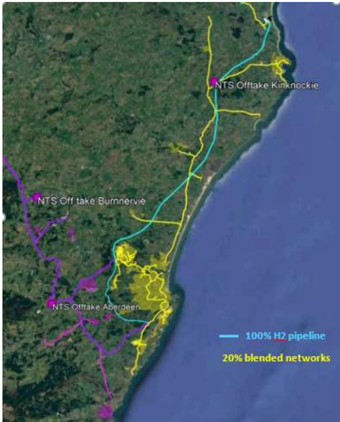
Image 4 shows the development of hydrogen within the gas network. This includes the construction of a hydrogen Pipeline as part of the Aberdeen vision project as well as 20% network blending into the existing gas network.
